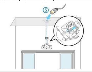
**Step 4**: Connect the Cat5 cable through the tubes of the drop pole.
