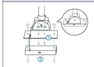
**Step 1**: Attach the mounting plate to the drop pole using the internal screws, then attach the counter to the mounting plate using the external screws.
