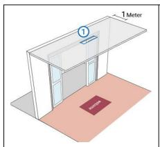
Step 1: Determine the mounting location (ideal height: 2.8m – 3.5m), cut the hole of camera space for installing the mounting plate (264mm x 70 mm)
