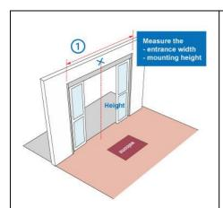
Step 1: Determine the mounting location (ideal height: 2.8m - 3.5m), calculate the total counter required using FootfallCam Calculator
