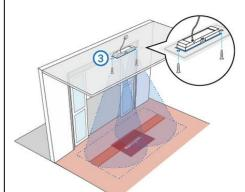
**Step 3**: Mount the plate with camera on the wall with 2x screws and wall plugs.
