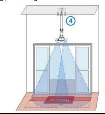
Step 3: Mount the drop pole onto the ceiling.
