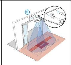
Step 3: Mount the bracket on the wall with 2x screws and wall plugs.
