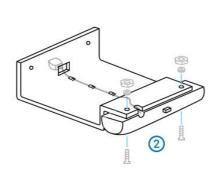
Step 2: Attach the counter to the bracket with 2x screws, nuts and washers.
