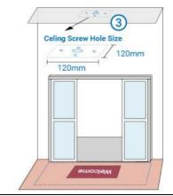
**Step 2**: Determine the mounting location and drill **(5)** holes for installing the drop pole. The holes should be drilled within **(120mm x 120mm)**
